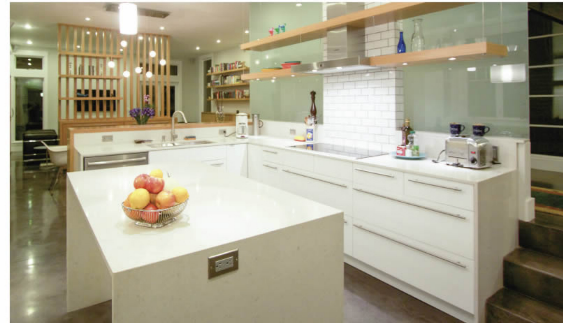
The sleek, open kitchen features an energy-saving Bosch 800 36-inch induction electric range with speed boost technology that heats up water twice as fast as a conventional stove. Pure white, sustainably manufactured Caesarstone quartz counter tops are both beautiful and practical; the non-porous surface prevents mold and microbes, and is low-maintenance to decrease detergent usage.
